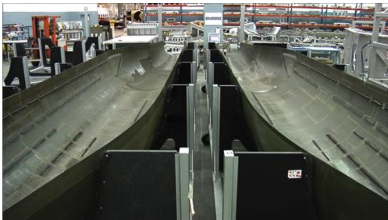
HondaJet – unitized composite fuselage
