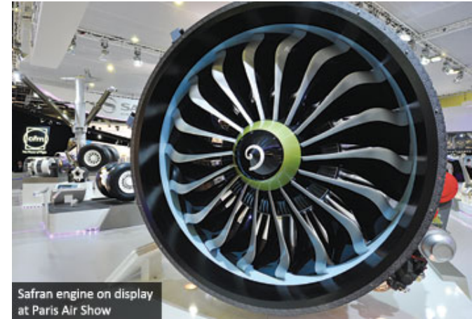
Safran engine on display at Paris Air Show CFM LEAP engine – Resin transfer molded fan blade
